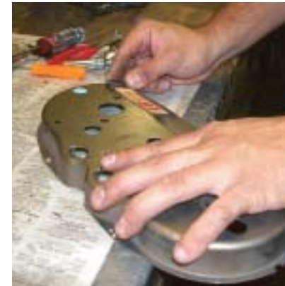
The Product Assembly Broadcast Label is removed with a razor blade and carefully preserved for reinstallation later. The ink stamp is covered with tape to preserve during the restoration process.
