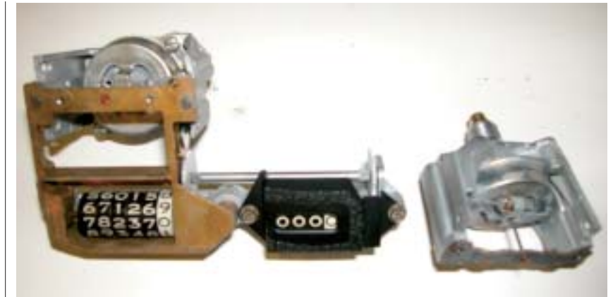
Here are the rebuilt speedometer and tachometer assemblies. After reassembly is complete, magnets are "charged." Restored faces and pointers are installed and units are attached to a special calibration machine that's been carefully maintained, since such machines have not been manufactured since the '60s.
