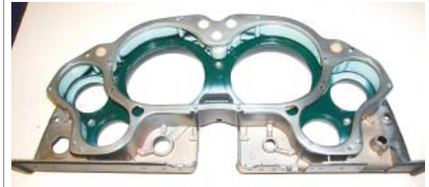
The internal part of the housing is specially painted to ensure original reflective qualities when the cluster is illuminated. The lens retainer plate is repainted black in front and two-tone green per factory patterns to assist with illumination.
