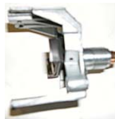
The worn bushings on the speedometer and tachometer frames are removed and replaced with new bushings. Shown is a view of a restored tach/speedometer frame after bushing installation.
